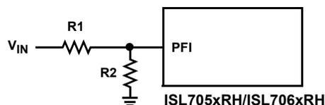
FIGURE 14. CUSTOM  $V_{TH}$  WITH RESISTOR DIVIDER ON PFI
