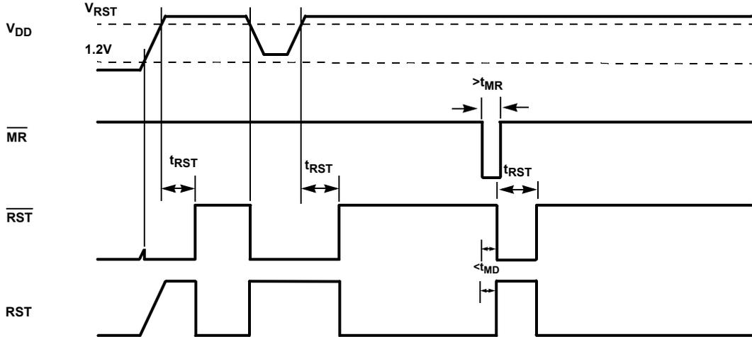
FIGURE 3. RST, RST-bar, MR-bar AND WDO-bar TIMING DIAGRAM
