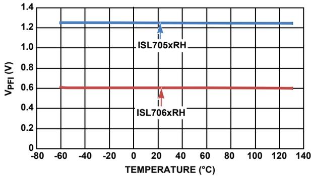
FIGURE 7. V<sub>PFI</sub> vs TEMPERATURE
