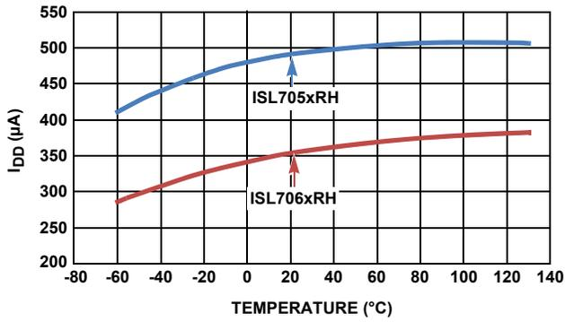
FIGURE 5. I<sub>DD</sub> vs TEMPERATURE
