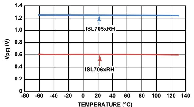
FIGURE 2. PRECISION THRESHOLD DETECTOR TEMPERATURE CHARACTERISTICS CURVE
